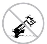
Use extreme care and slow speeds while driving the machine in stowed position across uneven terrain, debris, unstable or slippery surfaces and near holes and drop-offs.
